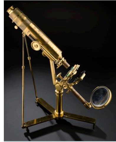
A 19th-century microscope featuring an achromatic lens
